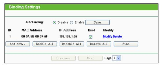
Figure 4-62 Binding Setting
