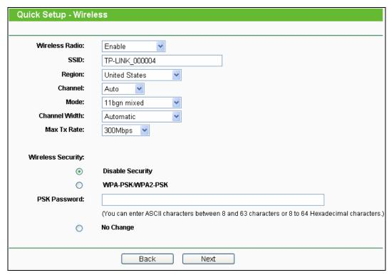
Figure 3-9 Quick Setup – Wireless
