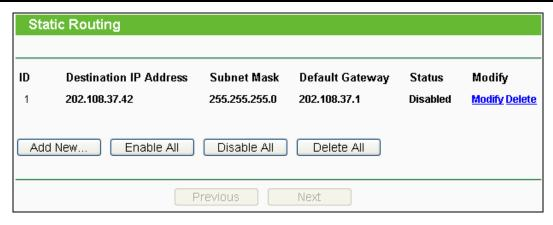
Figure 4-55 Static Routing
